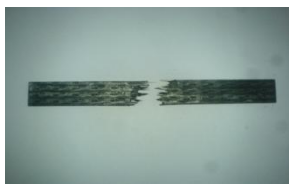
Fig. 13 Broken specimens in Flexural Test
