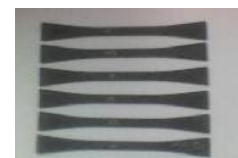
Fig. 7 Tensile test specimen geometry as per ASTM C1275 standards Fig.8 Tensile test specimens
