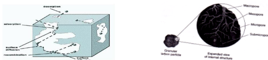
FIG.1. Macropore, mesopore, micropore and submicropore adsorption sites on activated carbon.
