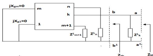
Fig 1. Thevenin's Impedance of Load Bus k.
