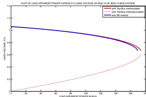
Fig 7. At Bus 14 of IEEE-14 Bus system
