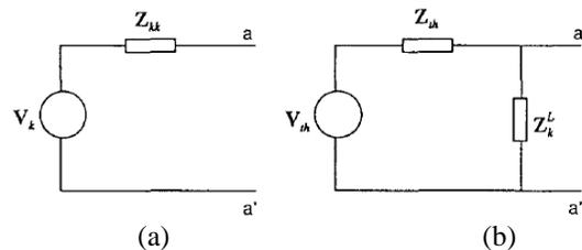
Fig. 2. Thevenin's Equivalent Circuits of Load Bus k
