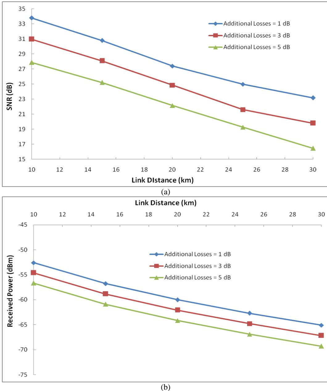
Figure 6 (a) SNR versus link distance (b) Received power versus link distance for different additional losses
