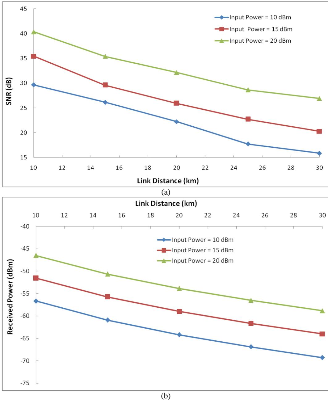
Figure 4 (a) SNR versus link distance (b) Received power versus link distance for different input power levels
