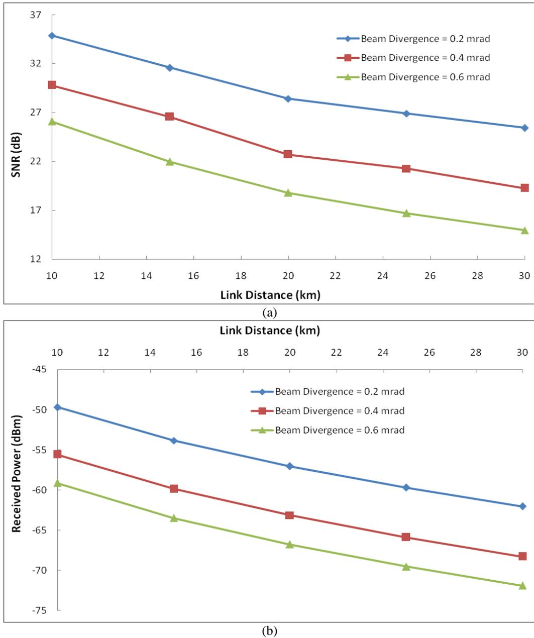
Figure 5 (a) SNR versus link distance (b) Received power versus link distance for different beam divergence angles
