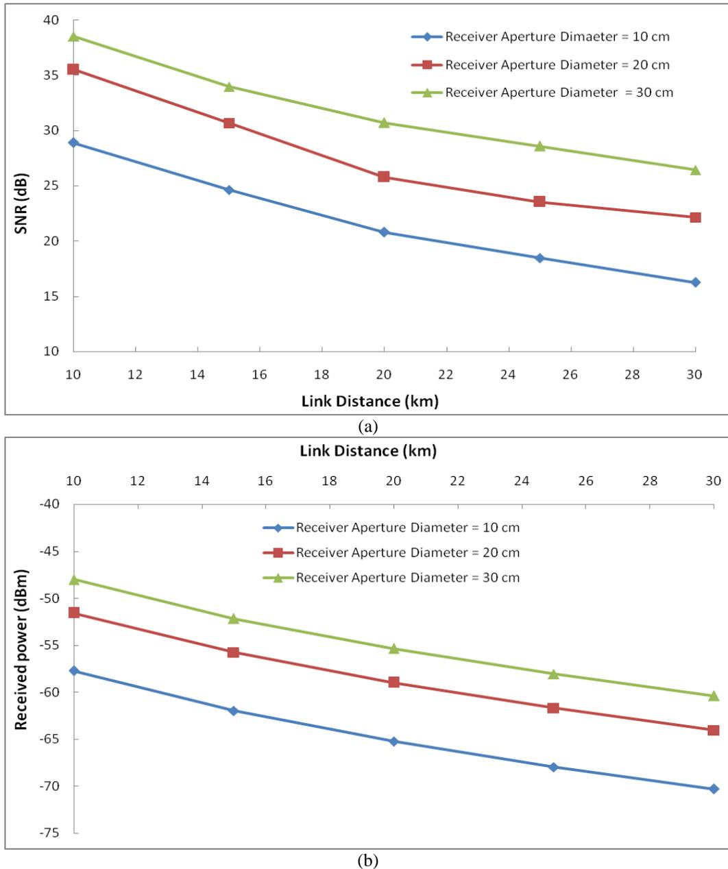
**Figure 3** (a) SNR versus link distance (b) Received power versus link distance for different receiver aperture diameter
