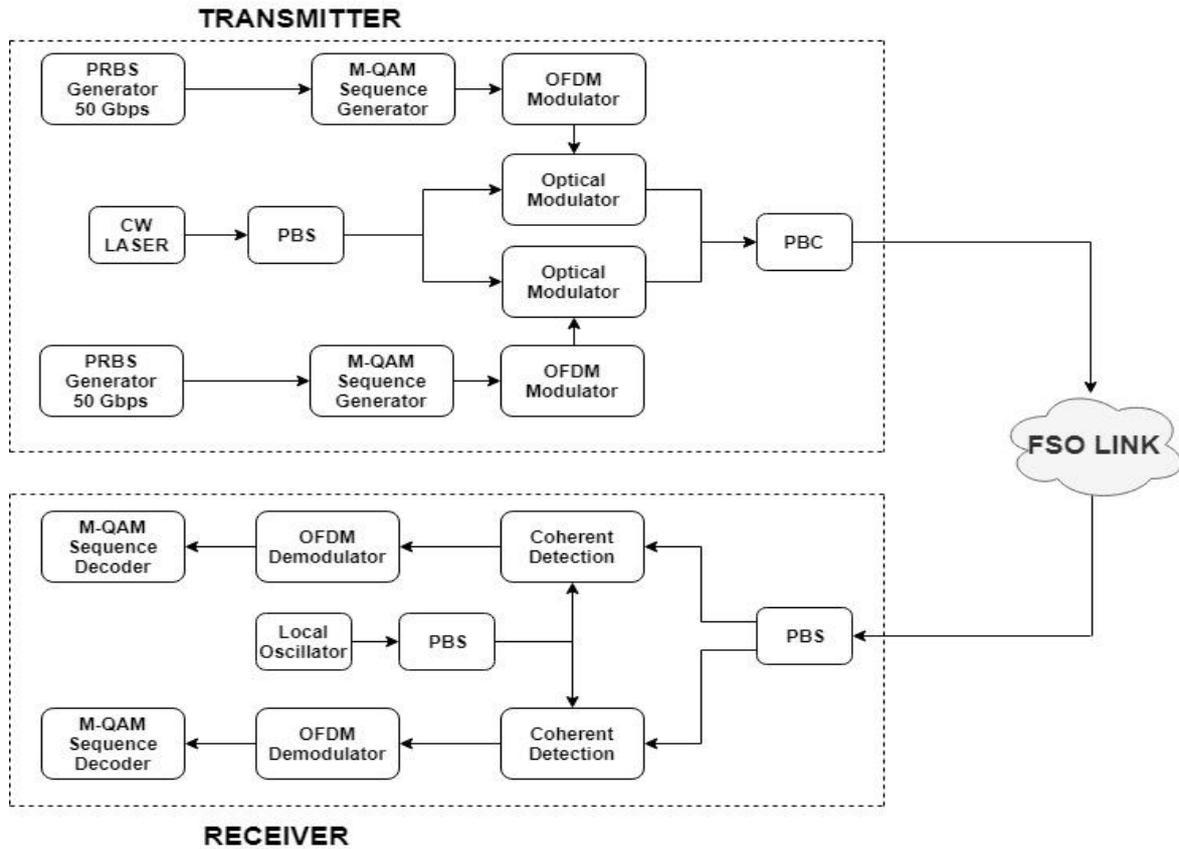
Figure 1 Proposed FSO system with PDM-CO-OFDM techniques
