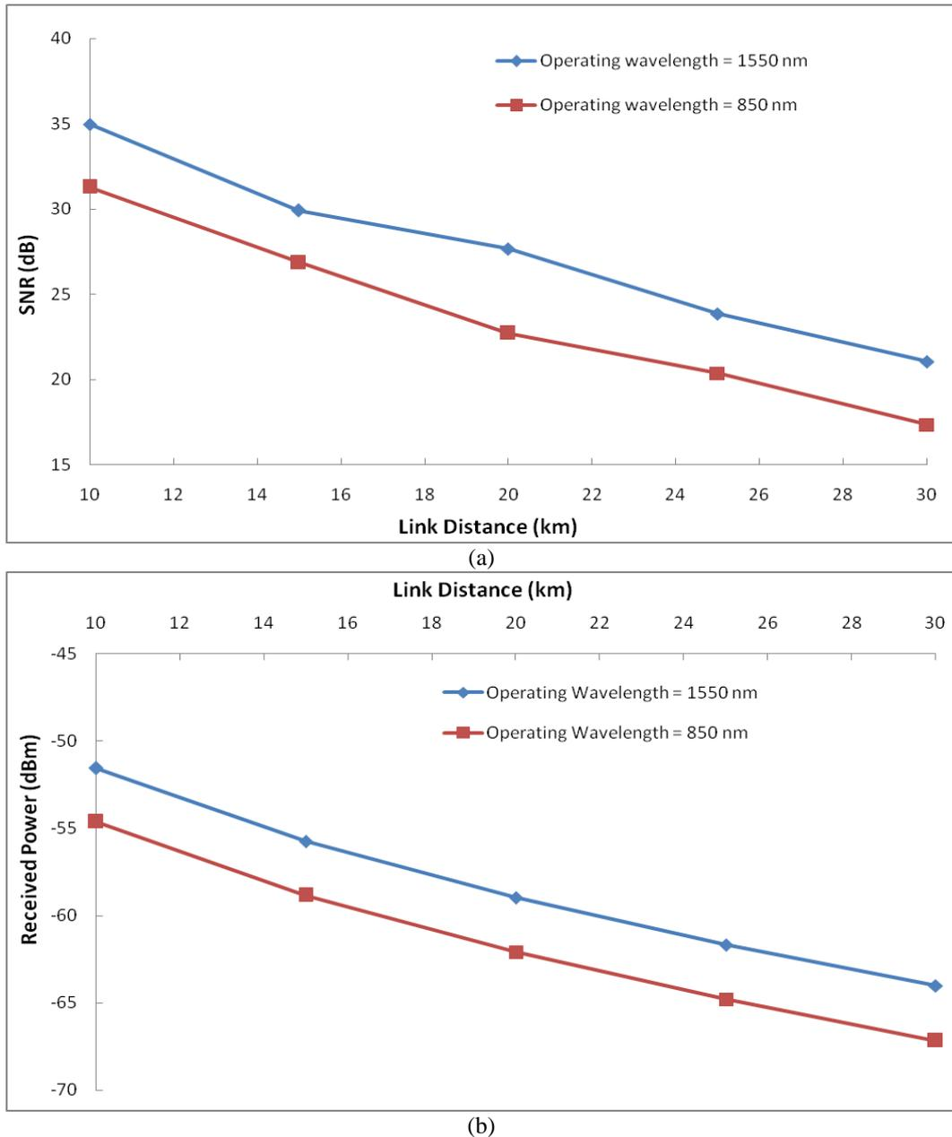
Figure 2 (a) SNR versus link distance (b) Received power versus link distance for different operating wavelengths
