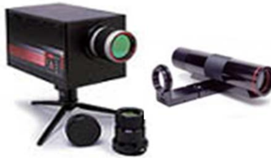
Figure 6. The thermocamera DeltaTherm 1560, and the zoom for high spatial resolution.
