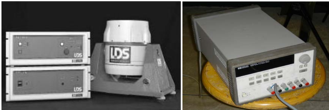
Figure 4. The shaker LDS 650, its amplifier 1000 PA (on the left), and the HP voltage generator.
