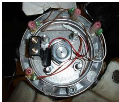
Figure 3. The four markers and the battery on flange.
