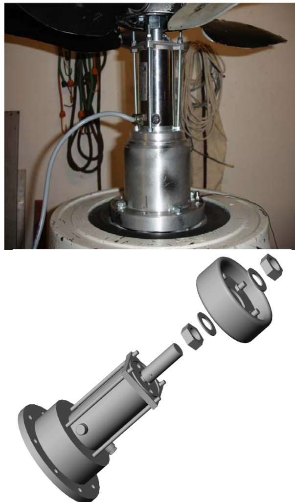
Figure 5. The test bench assembled on the shaker, and the CAD model.
